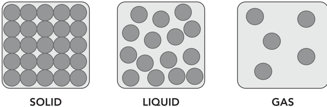
*Figure 1.1. Arrangement of atoms in different states of matter.*
