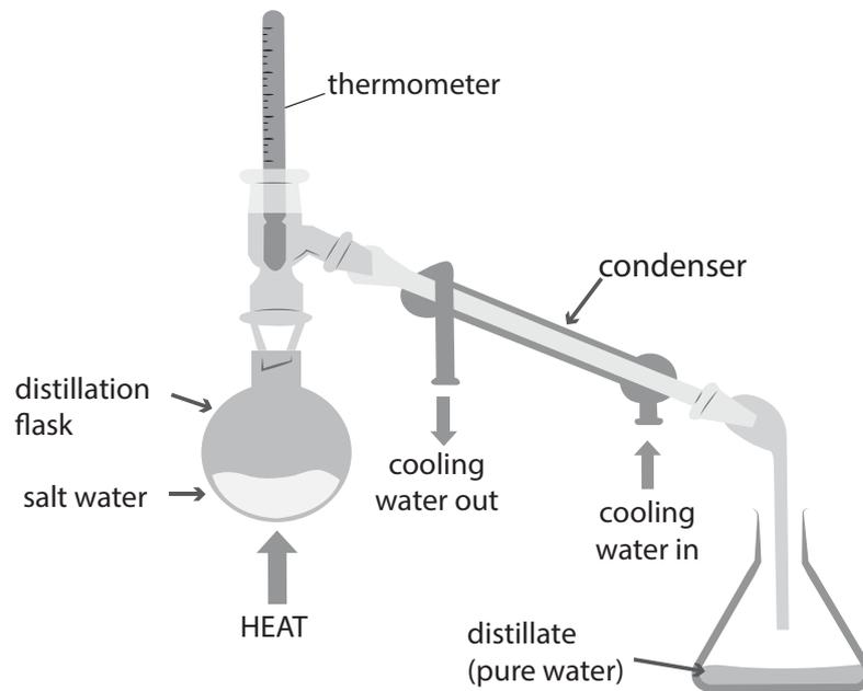
*Figure 1.8. Separation of salt and water can be done in two ways: **evaporation** produces water vapor which is released to the atmosphere, while **distillation** involves collection of condensed water vapor (returning to liquid state). Salt remains in the original container in both processes.*
