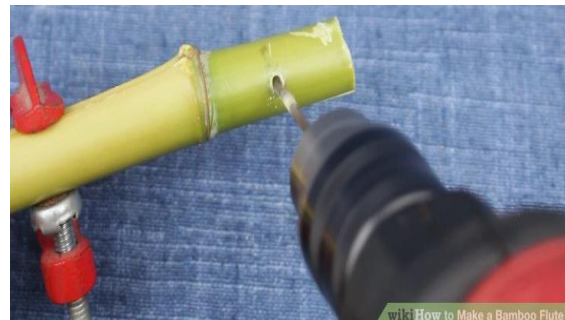
Clamp the bamboo down and begin to drill the embouchure.
