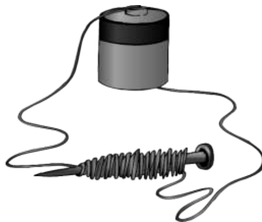
Figure 2. A simple electromagnet
