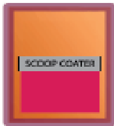
4.) Coat screen with Emulsion and Dry thoroughly
