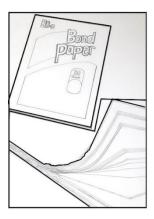
A bond paper (flat finish, 17x22) of substance 20 has a caliper of **thirty-five ten thousandths** while that of substance 24 has **four thousandths** caliper.
