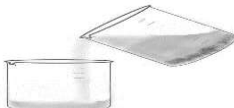
Figure D Decanting water with insoluble materials into the other container
