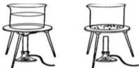
Figure E Evaporation is used to separate already dissolve solids.
