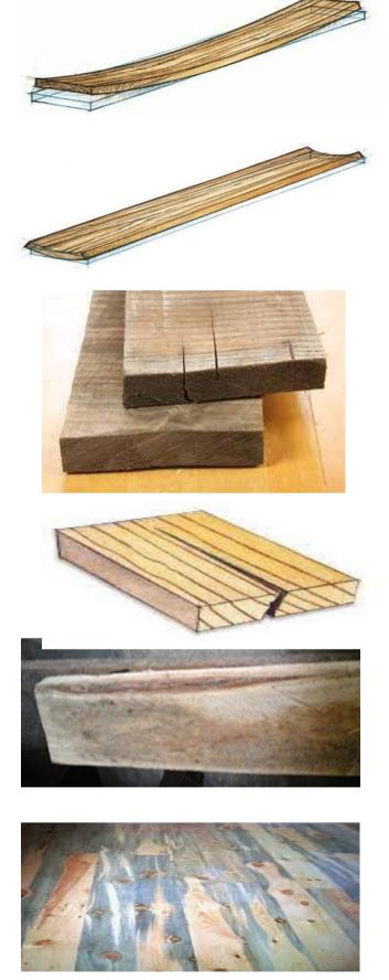
**Machine Burn** A darkening of the wood due to overheating by the machine knives or rolls when pieces are stopped in a machine.
