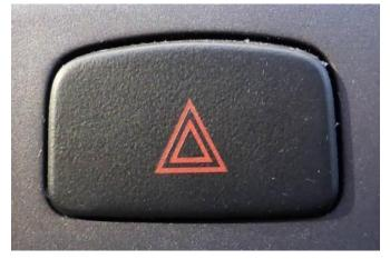
A device operated by the driver to indicate a vehicular hazard by flashing all signal lights together.
