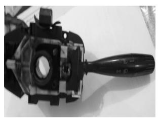
Late model vehicles combine switch controls into a single column mounted switch assembly so that the driver has ready access to systems such as windshield wipers and washer, turn signals, and headlights. These are all designed within a single multi-function switch so that the driver is able to keep his hands on the steering wheel during adverse weather or driving condition that would require the use of this system.
