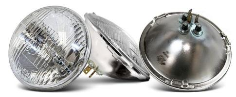
b. Semi-sealed beam type headlight- This type of headlight allows bulb replacement unlike in the sealed beam headlight. Since the bulb alone can be replaced, it is not necessary to replace the whole headlight assembly. This type is commonly used by modern vehicles.
