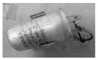
An automatic-reset circuit breaker used in directional signal and hazard warning circuits. When damaged, signal lights won't flash or lights steadily.
