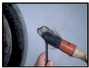
Brushing or dipping the holddown into the solution will neutralize the formed rust/corrosion.
