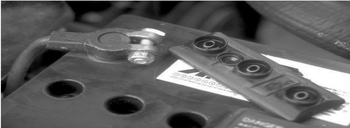
A battery with removable cell caps.
